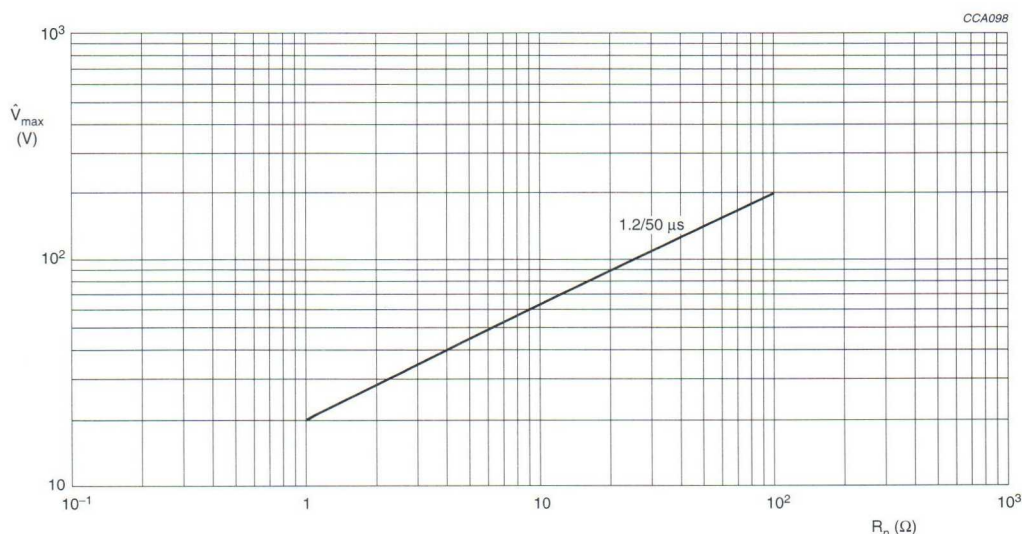
Fig.2 Maximum permissible peak pulse voltage without failing to 'open circuit' in accordance with DIN IEC 40 (CO) 533.
