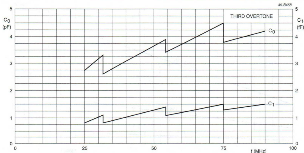
Fig.9 Motional capacitance C_1 and parallel capacitance C_0 as a function of resonance frequency, for crystals in 12 mm product length (involving large quartz blanks).
