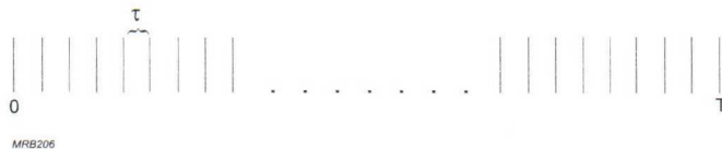
Fig.3.7 The probability of a photon arriving during the interval \tau is p = \tau/T
