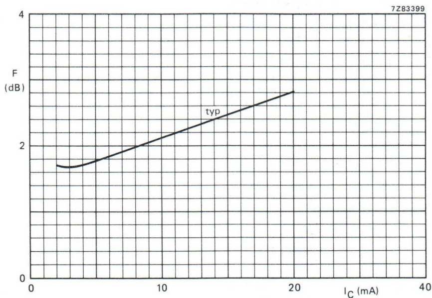
Fig. 13 V_{CE} = 10 V; f = 800 MHz; Z_S = \text{optimum} ; T_{\text{amb}} = 25 °C; typical values.
