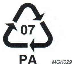
Fig.8 Other plastics. The acronym of the plastic is put under the recycling symbol. In this example: PA = polyamide.
