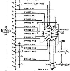
C<sub>1</sub>: 25 pF, 20%, 600 volts (dc working), ceramic disc C<sub>2</sub>: 50 pF, 20%, 600 volts (dc working), ceramic disc C<sub>3</sub>: 100 pF, 20%, 600 volts (dc working), ceramic disc C<sub>4</sub>: 250 pF, 20%, 600 volts (dc working), ceramic disc C<sub>5</sub>: 500 pF, 20%, 600 volts (dc working), ceramic disc C<sub>6</sub>: 100 pF, 20%, 1000 volts (dc working), ceramic disc C<sub>6</sub>: 100 pF, 20%, 1000 volts (dc working), ceramic disc
