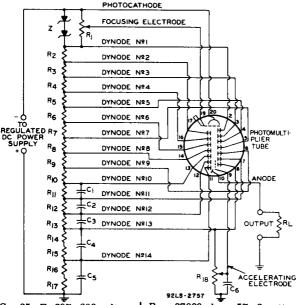
C<sub>1</sub>: 25 pF, 20%, 600 volts (dc working), ceramic disc C<sub>2</sub>: 50 pF, 20%, 600 volts (dc working), ceramic disc C<sub>3</sub>: 100 pF, 20%, 600 volts (dc working), ceramic disc C<sub>4</sub>: 250 pF, 20%, 600 volts (dc working), ceramic disc C<sub>5</sub>: 500 pF, 20%, 600 volts (dc working), ceramic disc C<sub>6</sub>: 100 pF, 20%, 1000 volts (dc working), ceramic disc C<sub>8</sub>: 5 megohms, 20%, 1/2 watt, adjustable R<sub>2</sub> through R<sub>11</sub>: 22000 ohms,
